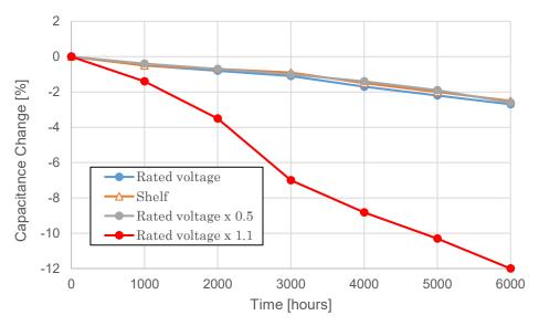
Fig. 24 Capacitance change when overvoltage is applied
