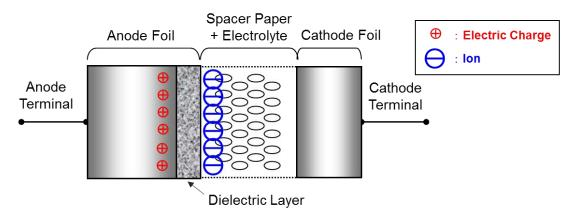
Fig. 1 Basic construction of an aluminum electrolytic capacitor
