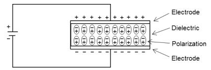
Fig. 29 Dielectric polarization during capacitor charging
