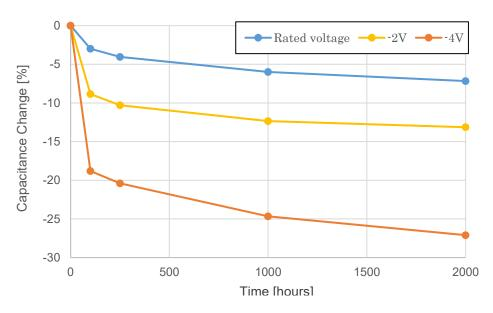
Fig. 25 Capacitance change when reverse voltage is applied
