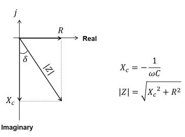
Fig. 9 Impedance and Loss angle of Capacitor
