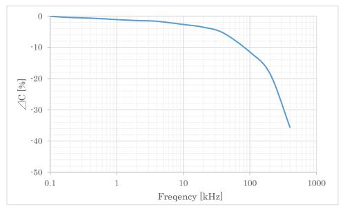
Fig. 17 The Frequency-response curve of capacitance
