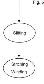
The master formed roll is then slit into individual rolls with specified width as per the specification.
