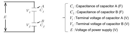
Fig. 26 Series capacitor connection
