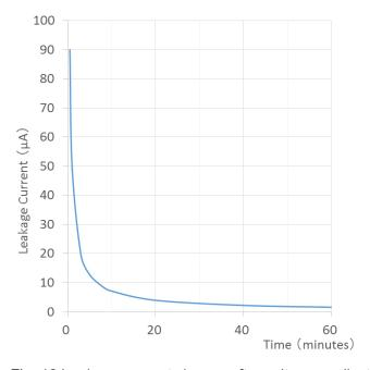
Fig. 12 Leakage current change after voltage application
