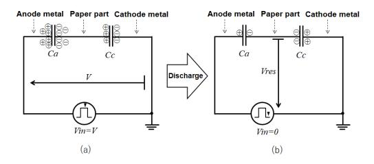
Fig. 23 The charge transformation on charge and discharge
