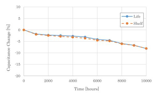
Fig. 18 Changes in capacitance with time at 105 °C
