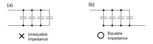
Fig. 28 Wiring for parallel connection of capacitors
