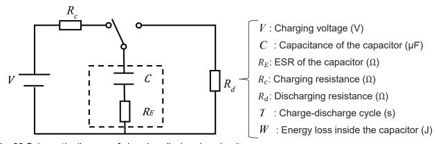
Fig. 22 Schematic diagram of charging-discharging circuit
