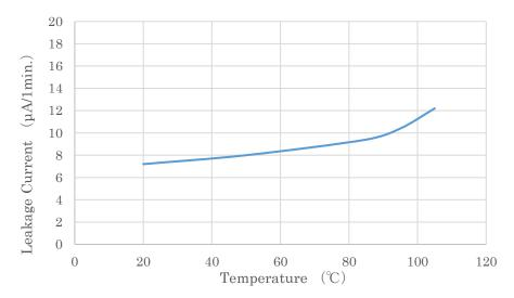
Fig. 16 Temperature Characteristics of leakage current
