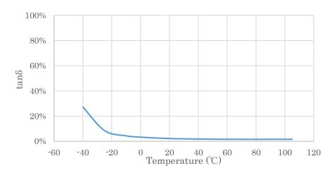
Fig. 15 Temperature Characteristics of the tangent of loss angle (tan  $\delta$ )
