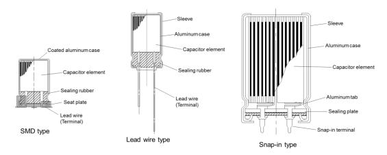
Fig. 3 Basic structure of aluminum electrolytic capacitor
