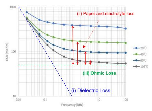
Fig. 11 ESR Characteristics of Aluminum Electrolytic Capacitor
