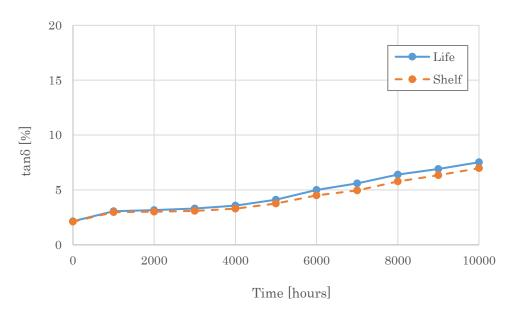
Fig. 19 Changes in tangent of loss angle (tan  $\delta$ ) with time at 105  $\,^{\circ}$  C
