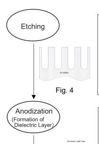
To obtain higher capacitance, surface area of aluminum foil for electrolytic capacitor increases through the etching process.
