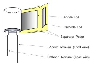
Fig. 2 Structure of aluminum electrolytic capacitor element
